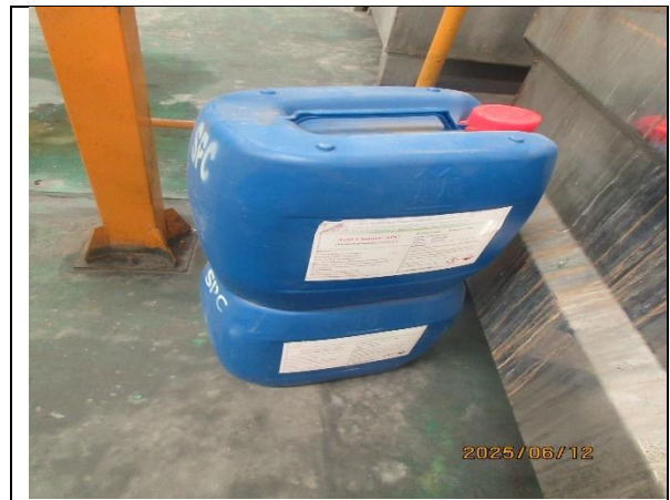
7.7 Lack of secondary container
